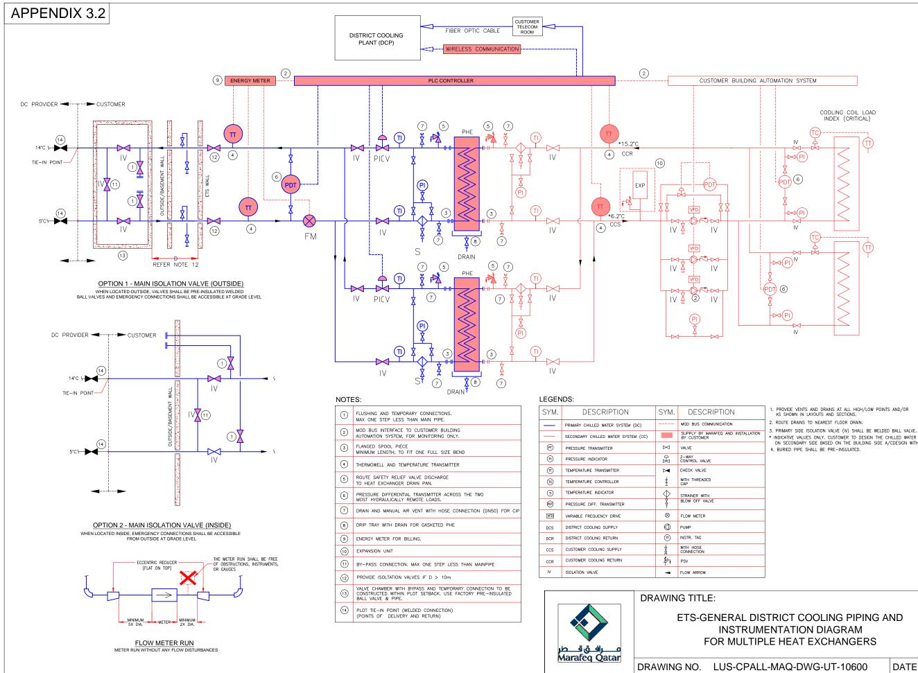
INDICATIVE VALUES ONLY, CUSTOMER TO DESIGN THE CHILLED WATER TEMPERATURES ON SECONDARY SIDE BASED ON THE BUILDING SIDE A/CDESIGN WITH DELTA T OF 9°C.
