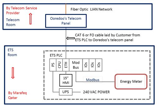
Figure 2 ETS Bulk meter schematic diagram
