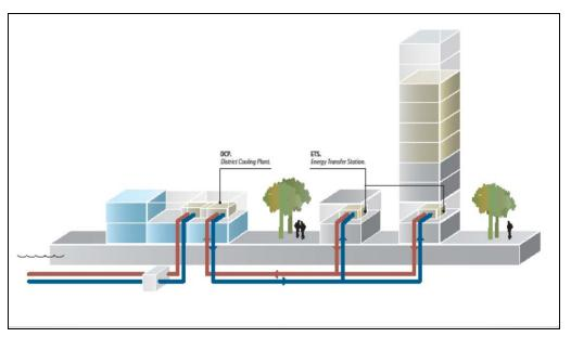
Figure 1: District cooling system general schematic
